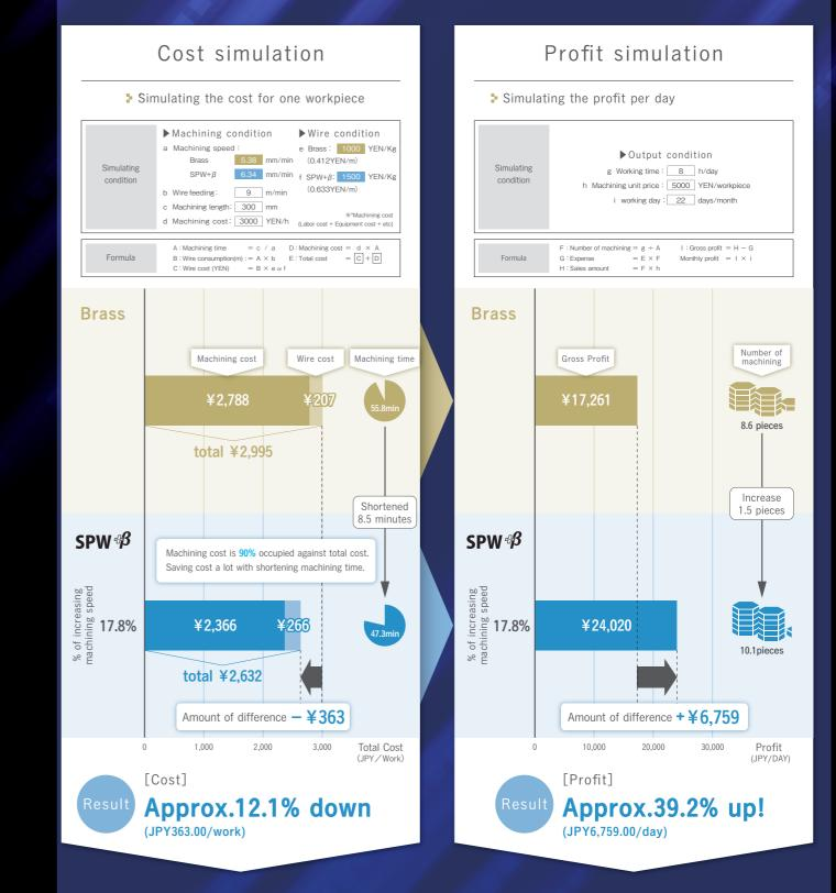
As reducing machining time, enable a costsaving and increasing of productivity, as a result, increasing 39.2% of profit (JPY148,703.00/month.)
