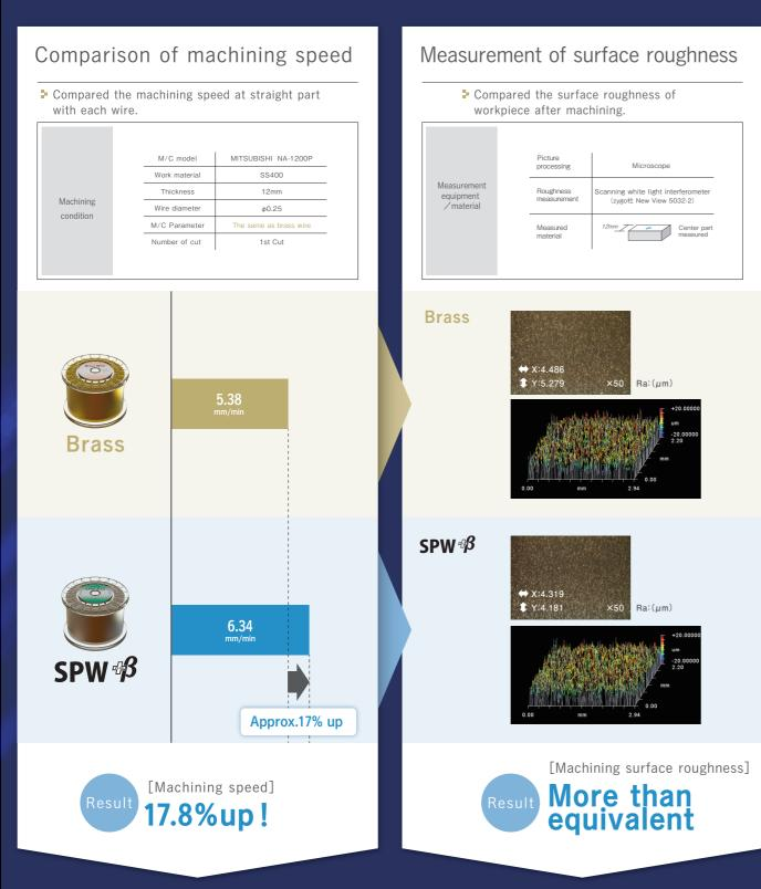
Just change the wire (No change of parameter), get increasing 17.8% machining speed. In addition, surface roughness doesn't degrade even increasing of machining speed.
